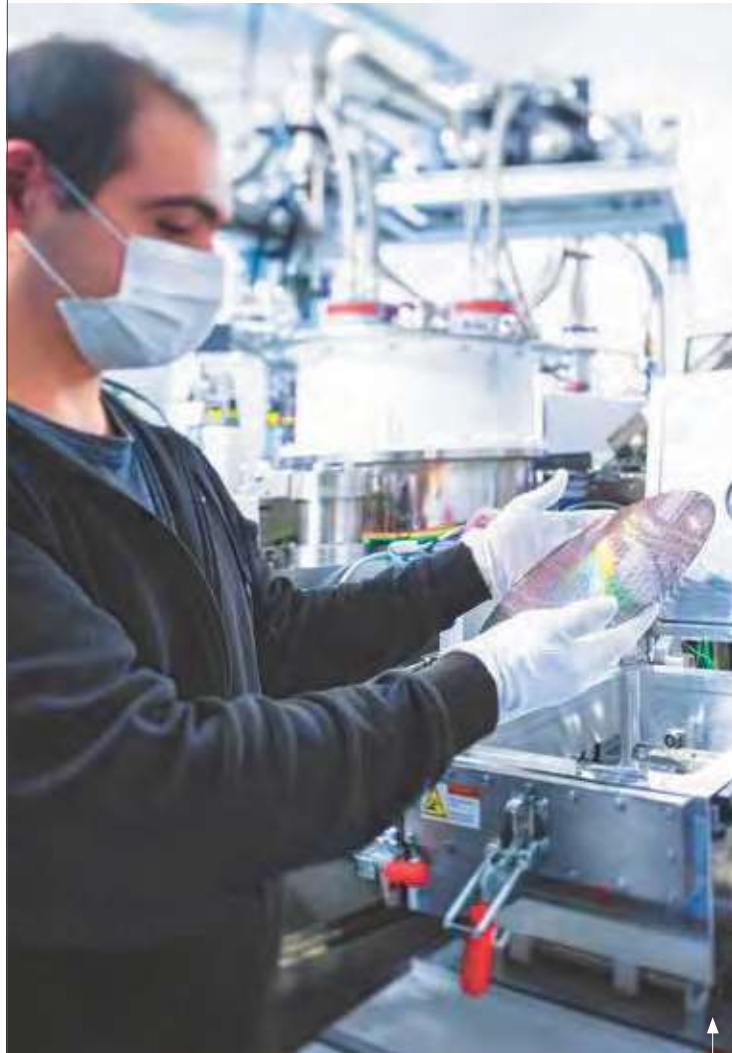
CRYOGENIC TEMPERATURE TEST BENCH FOR 300 MM INDUSTRIAL STANDARD WAFERS CARRYING CMOS TECHNOLOGY QUBITS, AT CEA-LETI
