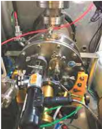
A VIEW OF THE DEUTERIUM IONS SOURCE ON THE GENESIS ACCELERATOR 14 . A NEUTRON BEAM (14 MEV) IS GENERATED BY THE NUCLEAR REACTION OF DEUTERIUM NUCLEI ON A TRITIUM TARGET. THE GENESIS INSTALLATION IS MAINLY USED TO TEST THE EFFECTS OF A SINGLE EVENT IN THE FIELD OF MICROELECTRONICS, ON DIAMOND OR SILICON WAFERS. ACCESS TO THIS UNIQUE INSTRUMENT IS INCLUDED IN THE PAC-G SERVICE FOR INDUSTRIAL STAKEHOLDERS.
