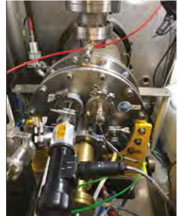
A VIEW OF THE DEUTERIUM IONS SOURCE ON THE GENESIS ACCELERATOR 14 . A NEUTRON BEAM (14 MEV) IS GENERATED BY THE NUCLEAR REACTION OF DEUTERIUM NUCLEI ON A TRITIUM TARGET. THE GENESIS INSTALLATION IS MAINLY USED TO TEST THE EFFECTS OF A SINGLE EVENT IN THE FIELD OF MICROELECTRONICS, ON DIAMOND OR SILICON WAFERS. ACCESS TO THIS UNIQUE INSTRUMENT IS INCLUDED IN THE PAC-G SERVICE FOR INDUSTRIAL STAKEHOLDERS.
