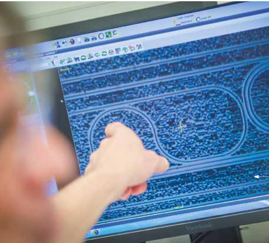
MICROSCOPE VIEW OF THE PHOTONIC MZI CIRCUIT DESIGNED AND PRODUCED AT CEA-LETI FOR ALCOHOL DOSE TITRATION
