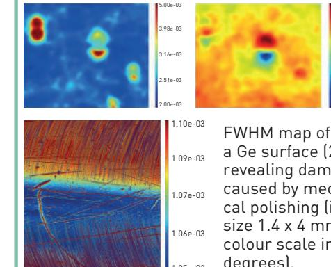
FWHM map of a Ge surface (220) revealing damages caused by mechanical polishing (image size 1.4 x 4 mm<sup>2</sup>, colour scale in degrees).
