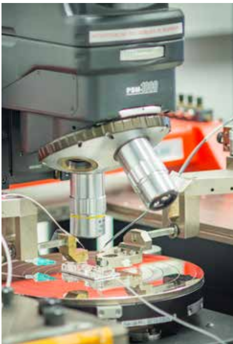
Above right, TESTING THE VERY FIRST PROTOTYPE OF A PHOTONIC SENSOR FOR ALCOHOL DOSE TITRATION © O.DEVISE/CEA
