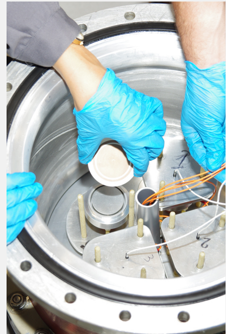
Fig: Photo of the measurement samples being placed in the platform © SuperGrid Institute
