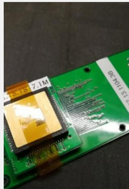
SRAM commercial memory set-up on a connecting PCB ready for irradiation at the ILL, the European neutron source for research, based in Grenoble ©Cern
