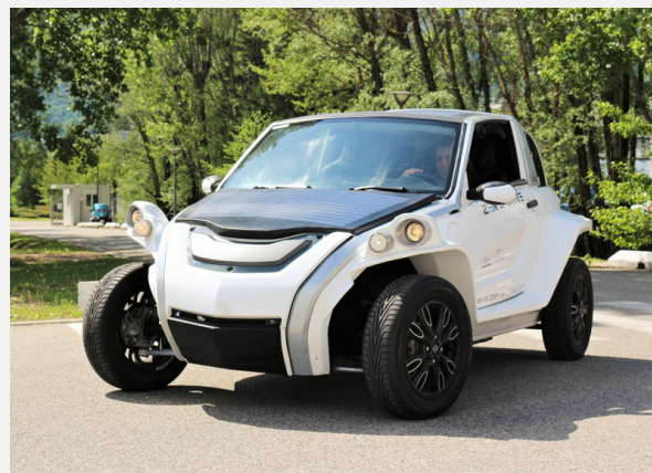
A first prototype of an electric car with integrated PV system. © CEA
