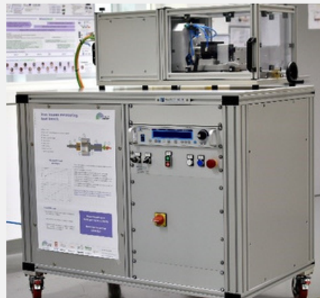
Iron losses measurement test © IRT Saint Exupéry
