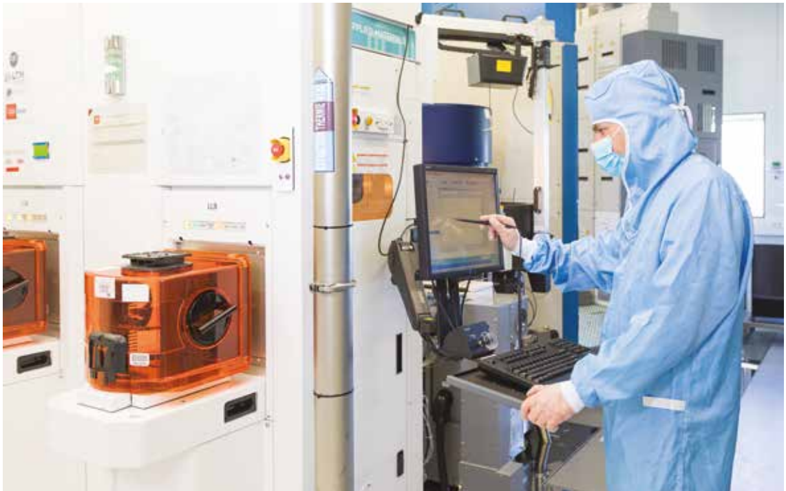
↑ Mickael Martin, microelectronics engineer at the CNRS. MOCVD III-V (Metal-Organic Chemical Vapor Deposition) epitaxy deposition platform control console – Operated by the Microelectronic Technologies Laboratory (CNRS-UGA) and CEA-Leti, this machine was used to develop industrial standard red LEDs.
