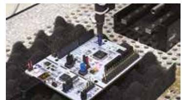
↑ Classic setup for electromagnetic emanation recording (target being tested is a Cortex M4 32-bit microcontroller). © CEA
