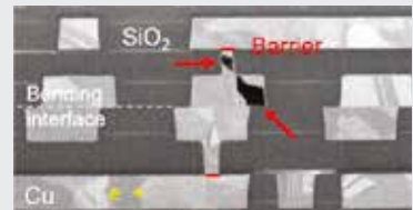
↑ Electronic imaging of hybrid bonding failed structure (void in Cu material) after an accelerated electromigration test: (presented at IRPS 2023 Conference)
