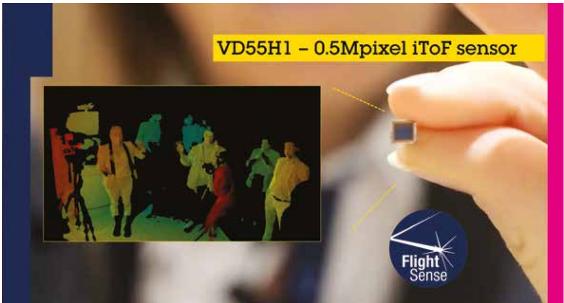
↑ STMicroelectronics recently launched the VD55H1, a low-noise, low-power indirect time-of-flight (iToF) sensor array of 672 x 804 pixels (0.54 Mpixels). © STMicroelectronics
