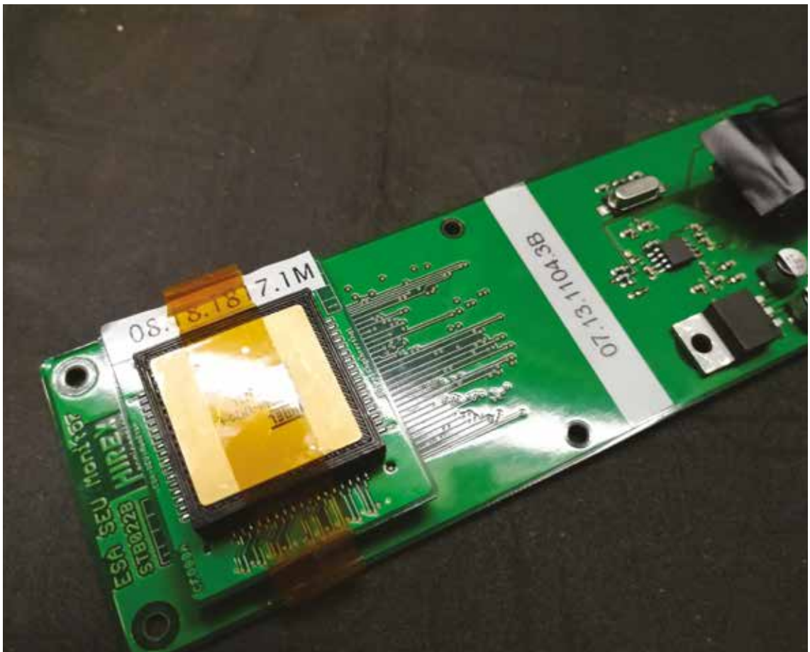
↑ SRAM commercial memory set-up on a connecting PCB ready for irradiation on the ILL D50 beamline. ©CERN
