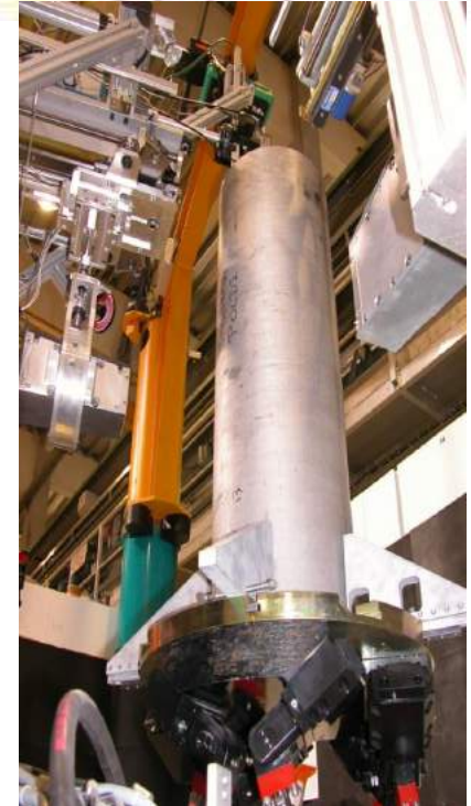
A 2 m Al billet being placed on the sample stage of an ILL instrument
