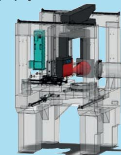
Neutron and X-ray testing environment. The Tomographs are supported by a granite table, for maximal thermal and vibrational stability.
