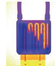
Neutron radiogram of a heat exchanger partially filled with water.
