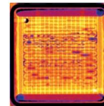
Part of the vapor generated as a byproduct in a fuel cell condenses into liquid water. Courtesy A.Morin CEA-Grenoble
