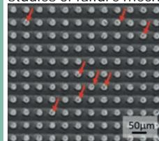
Slice image acquired from a flip-chip showing the interface between two dies. We can observe copper pillars in white and defects as black dots (some are highlighted by red arrows).
